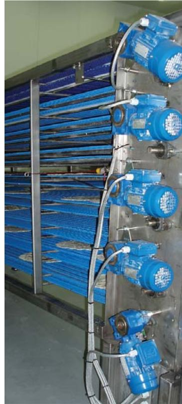
shafts for each of the conveyors were being driven by a system of chains and sprockets from one large geared motor, with very high torque. Frequent jams, caused by a dislodged pizza and the consequential build-up on individual conveyors resulted in broken drive shafts. Knock on effects were a halt to production and high maintenance costs as new, tailor-made drive shafts had to be specially machined to replace the broken ones – amounting to high annual maintenance costs of around €3,500.
