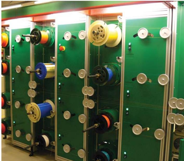
The new and highly innovative range of ComPo optical fibre and cable unwinders from Finnish company Compomec Oy, all feature Commander SK AC drives supplied by Control Techniques' local distributor SKS Control Oy.
