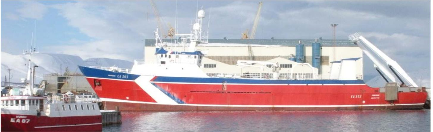
**One of the world's most advanced survey vessels features bow and stern thrusters powered by Control Techniques modular AC drives to achieve position accuracy of  $\pm$  one metre.**
