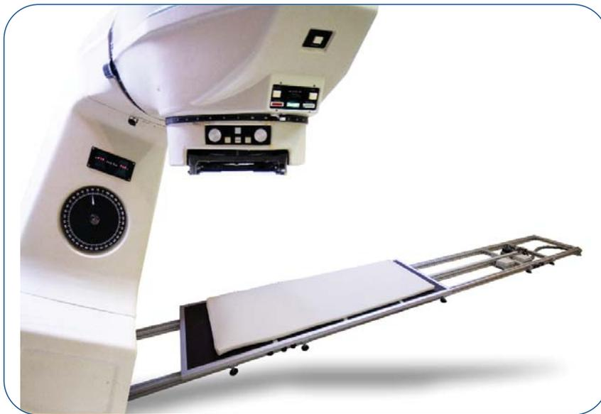
The original system was designed and built in 1989 by the maintenance department of the Institute of Oncology Ljubljana, and featured a DC servo drive for the control of the table movements. However, advances in radiation treatment led to the need for an upgrade to achieve better accuracy and improved reliability.
