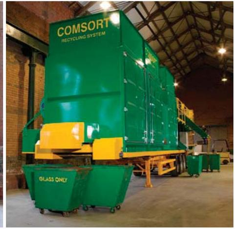
Mixed recyclables, entering the process via a feed hopper, travel up an elevated feed conveyor onto the apron conveyor, where operators manually remove large pieces of unrecyclable waste (masonry, toys, prams etc). Thereafter, initial separation of steel is facilitated using an overband magnet, and aluminium, using a high-performance eddy-current separator. All this is well-proven technology.
