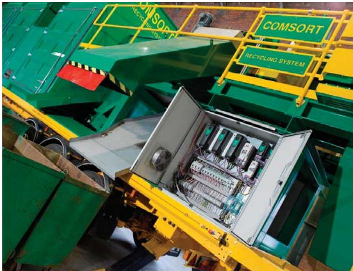
A new, commingled separation machine, designed and built by air technology specialists Tek-Dry of Bolton, offers a solution to a national shortage of good quality glass cullet, by eliminating glass pulverisation during the separation process. The 'Comsort' system uses new, patented, air technology to offer a revolutionary low impact separation system for commingled recyclables.
