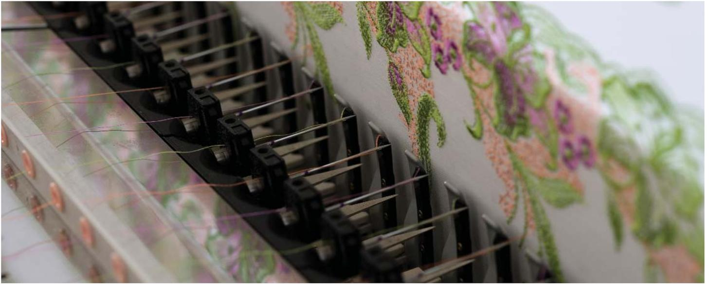
Machines can feature up to 32 axes, each controlled by the MultiAx / SLM Unimotor combination –the main axis being the feed; the needle, borer and shuttle axes being electrically slaved to this to maintain synchronisation. Frames can weigh up to 500 kg and movement of up to 5-mm is required in just 30 milliseconds!
