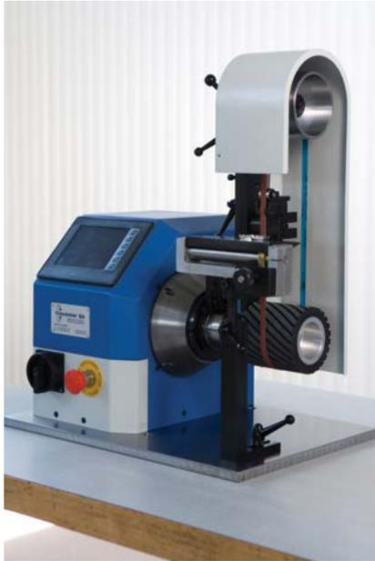
**Crevoisier SA of Les Genevez, Switzerland are a leading manufacturer of production machines for the high class watch making industry. They have recently launched The Universal C-5001 Lapping and Polishing Machine and at its heart is a Control Techniques 1.5 kW (400VAC) Commander SK running a 1.5 kW motor all controlled by a colour touch screen HMI panel.**
