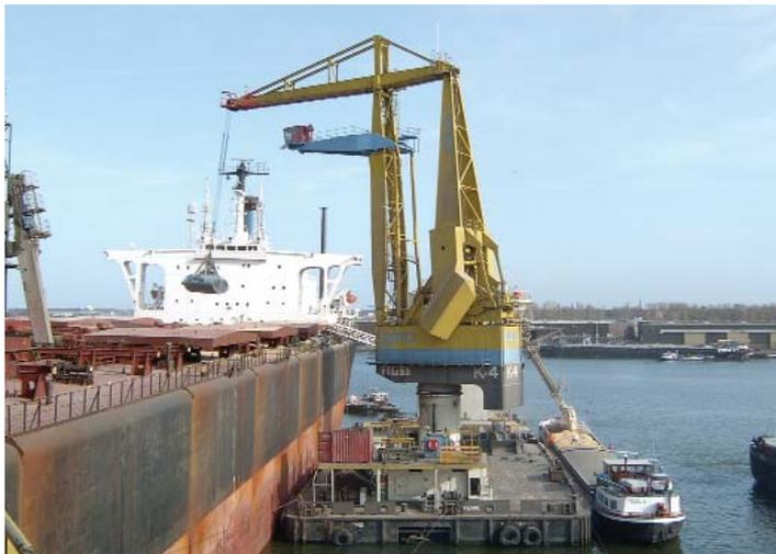
**Control Techniques' Drive Centre, the Netherlands has recently completed the retrofitting of four floating grab cranes. All four cranes, situated at Amsterdam, have the four-rope grab system and are mainly used for ship to quay bulk handling. Two of the cranes are rated at 16-tonnes and have been retrofitted with AC Unidrive variable speed drives, while the two larger 25-tonne cranes have a DC solution, with Mentor II DC drives.**
