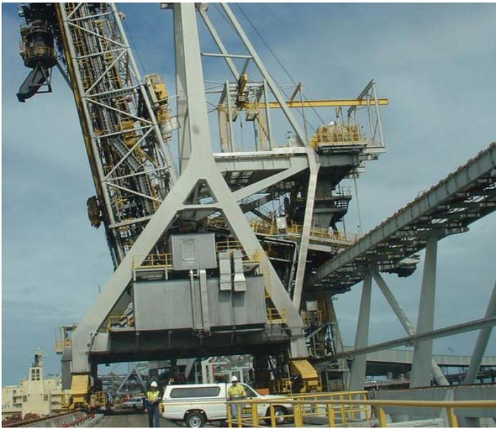
AC drives from Control Techniques feature on a new shiploader installed at the Dalrymple Bay Coal Terminal in the port of Hay Point, Queensland, Australia. The massive shiploader serves a total of 14 mines in Central Queensland including Blair Athol and is part of Babcock & Brown Infrastructures expansion plans.
