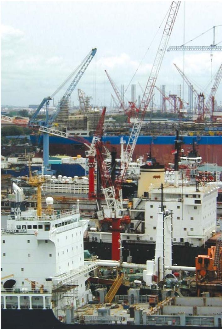
The unique constant load height feature makes the crane operation both easier and safer. The 30 kW luffing (jib) drive can lift the jib from horizontal (0°) up to 89°. This would normally change the height of the load above the ground. During cargo loading and unloading, there is a need to keep the load at a constant height. This is achieved by operator key selection, at which point the drives take-over.
