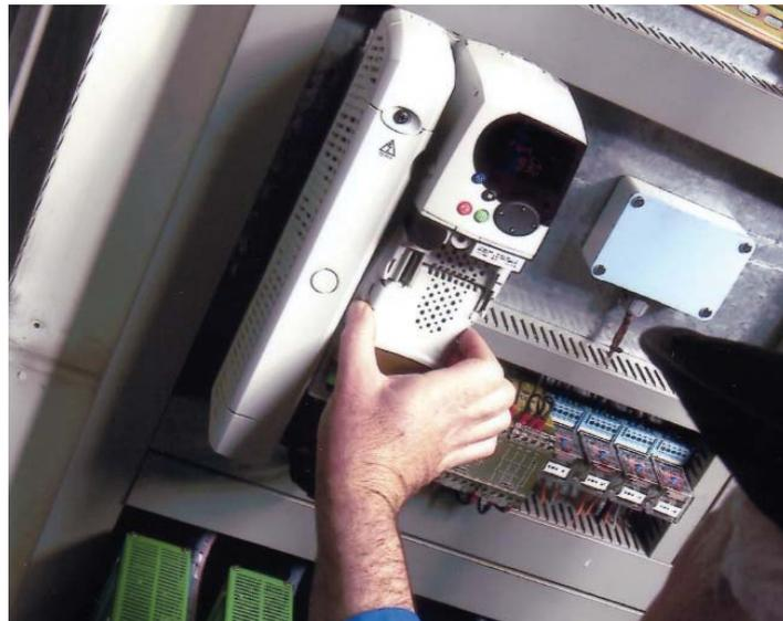
Six Control Techniques 'Maxi Maestro' high performance DC servo amplifiers were chosen for the control of the lane/crimping drives, another for the wrapper feeder whilst a 7.5 kW Unidrive SP powers the jaw drive, with its on-board SM application module provides the complete programming for the wrapping machine, eliminating the need for the PLC previously employed.
