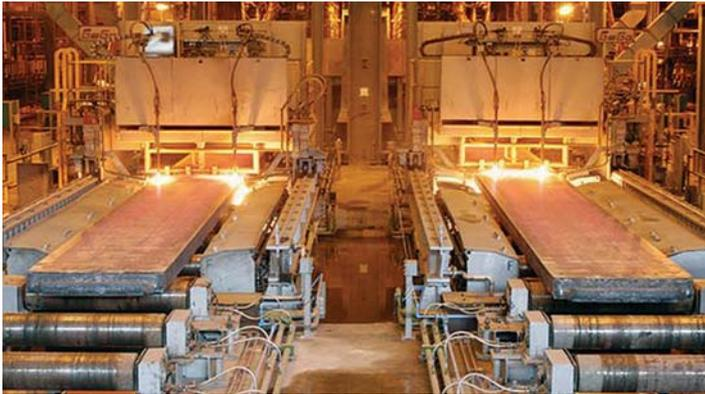
**Control Techniques drives feature on the latest continuous slab caster at Corus steelworks in Port Talbot, South Wales, controlling critical operations at the head of the line. The total output of the plant, anticipated to be 4.7 million tonnes in 2006, is dependent on drives from Control Techniques.**
