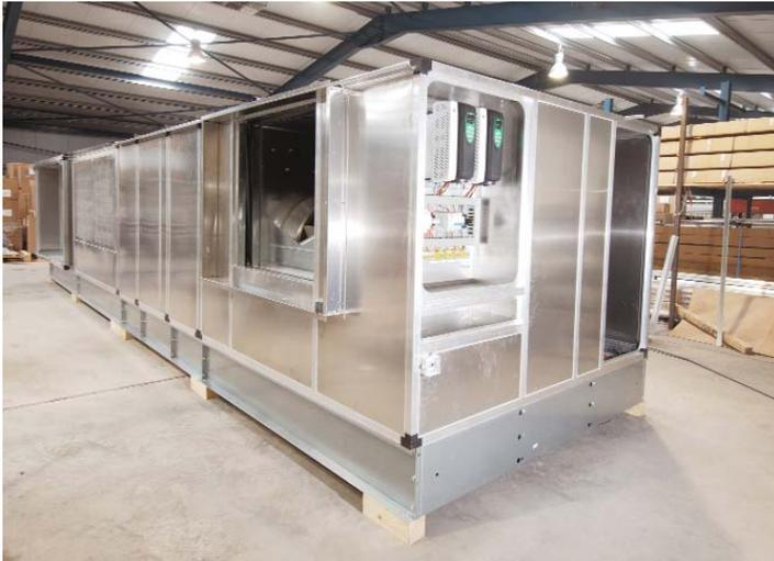
**Ireland's leading manufacturer of air handling units for heating, ventilating and air conditioning has standardised on AC variable speed drives from Control Techniques.**
